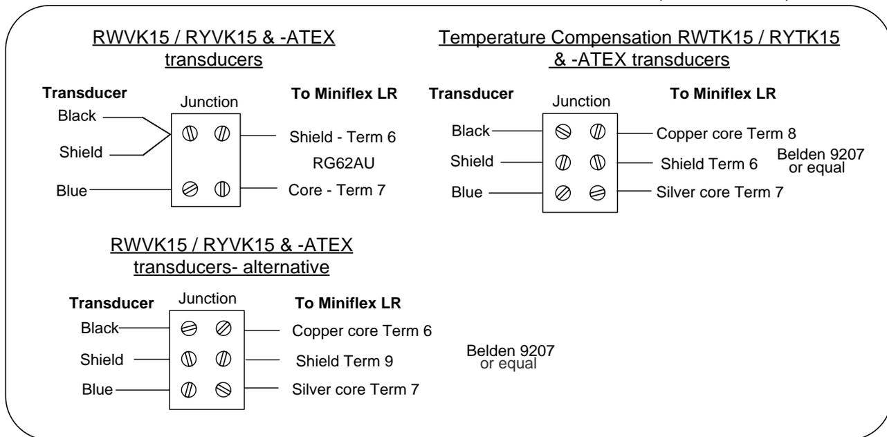
Figure 7: Transducer cable extension diagram
