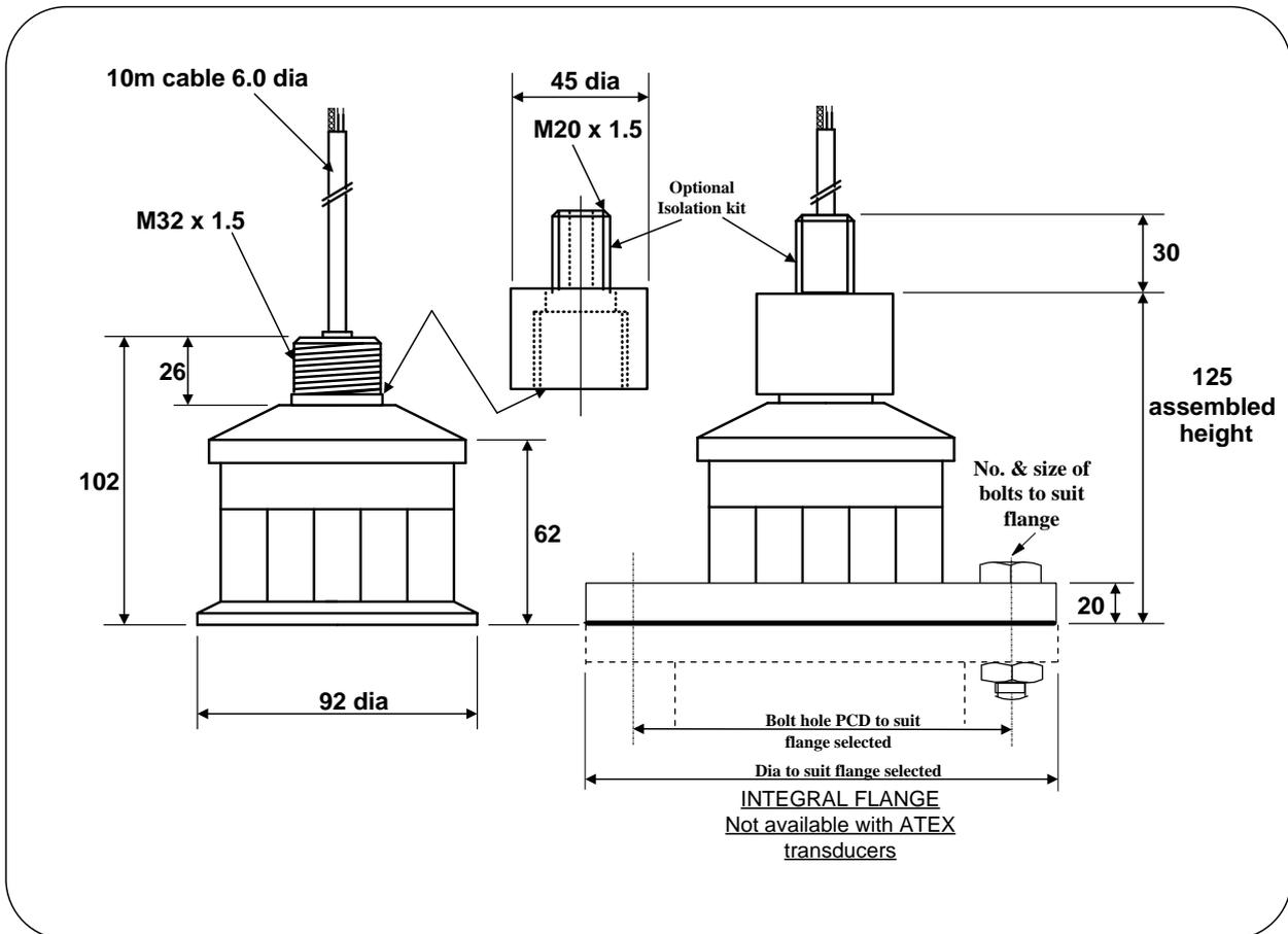
*Figure 4: Transducer dimensions*
