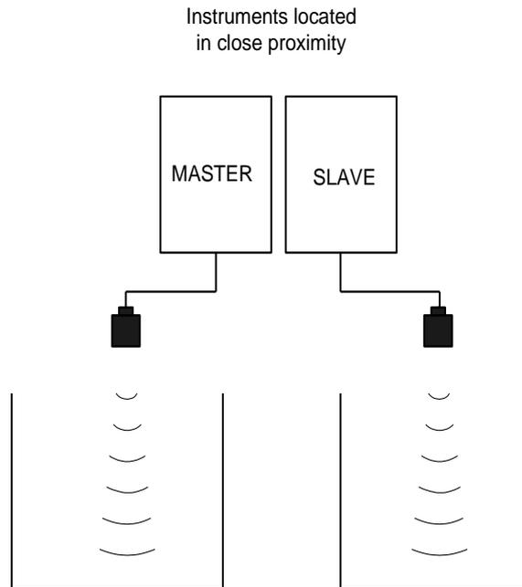
*Potential problem application with two instruments located close together.*
