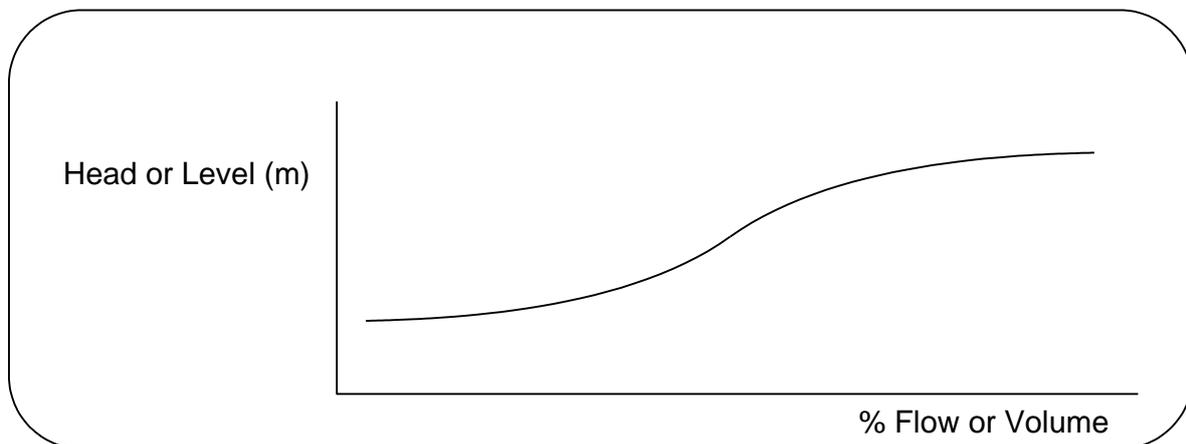
The profile data are input into Pr.6.1.8 for volume and Pr.7.1.8 for flow. The values can be displayed and changed as required.
