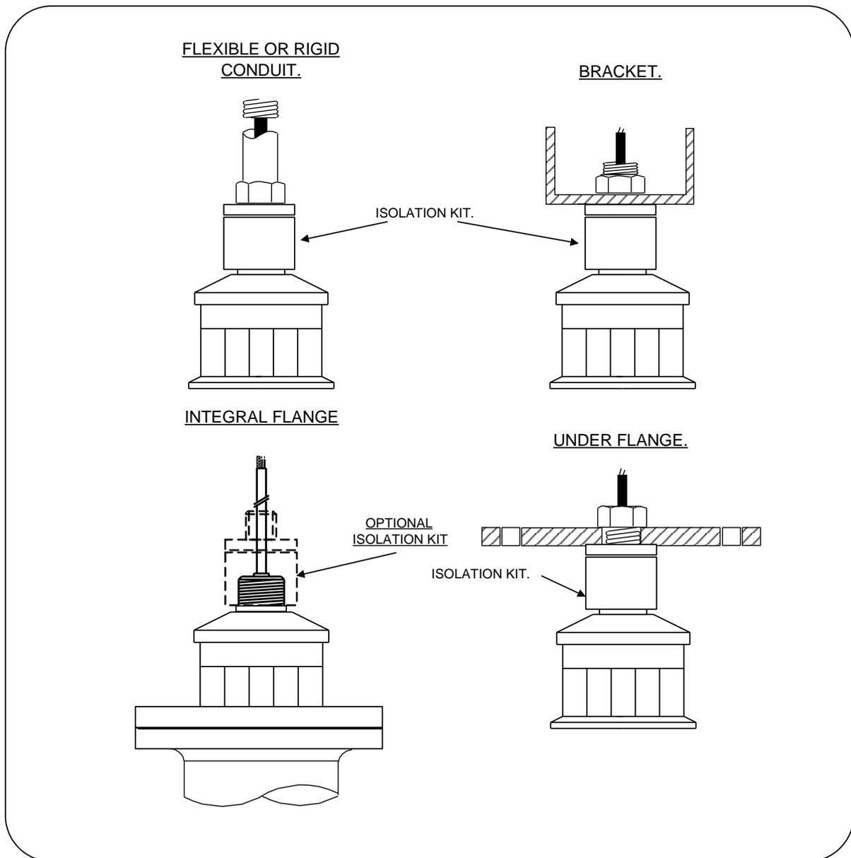
*Figure 5: Alternative mounting arrangements for transducers*
