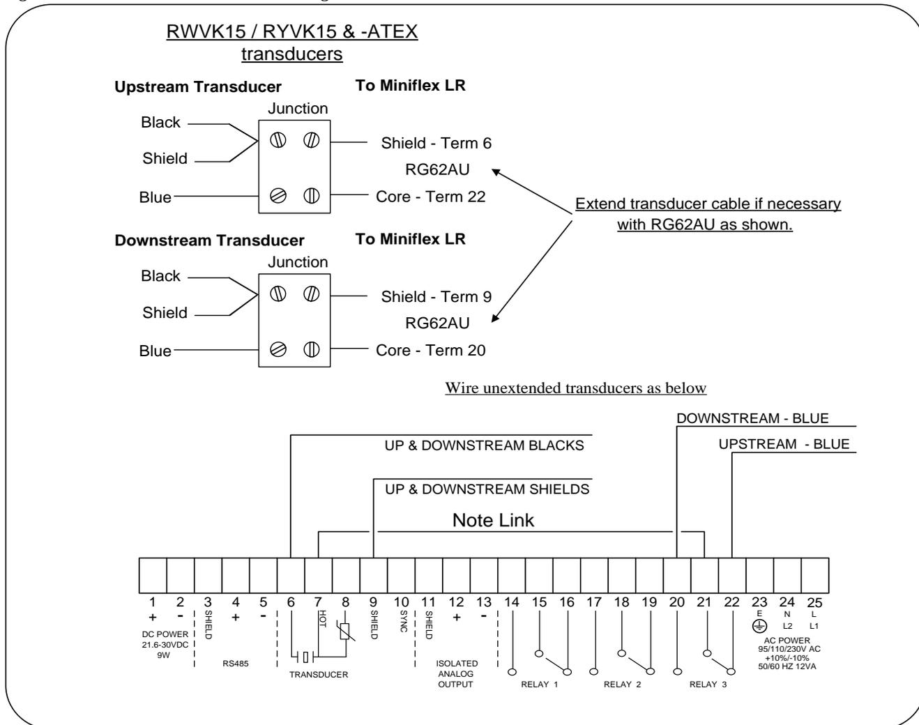
Figure 8: Transducer wiring for differential mode
