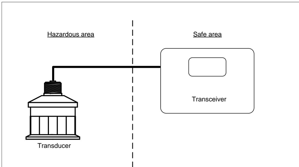
The installation must be in accordance with the applicable codes of practice and harmonized standards for Ex mb (encapsulated) equipment.
