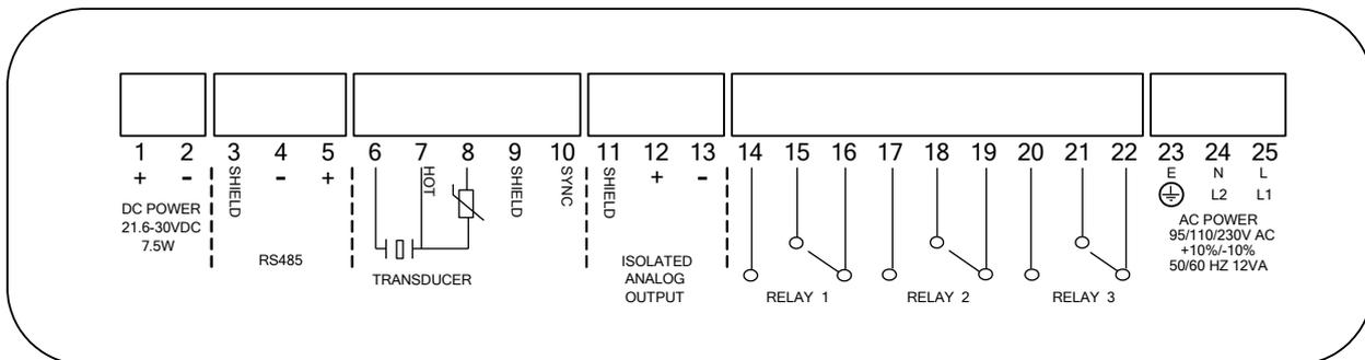
Figure 3: Wiring diagram label inside Miniflex LR terminal cover
