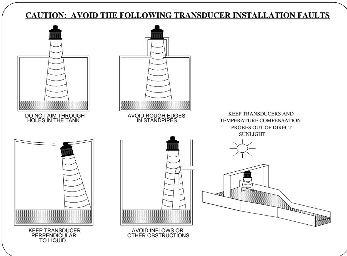
Figure 6: Transducer installation faults
