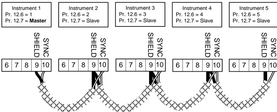
*Connection diagram for up to 5 instruments*
